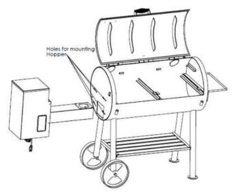
4 Slide the hopper all the way in until it contacts the grill side. Have the other person hold the hopper in place while you screw in a bolt and lock washer into each of the 4 mounting locations from the inside of the grill as shown below.
